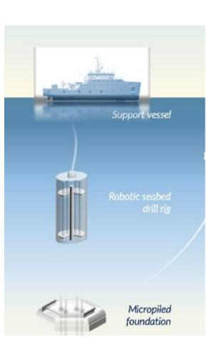
Install micropile anchors offshore (with load test)
