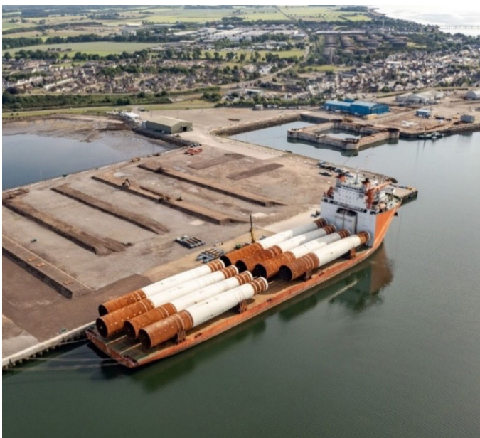
Moray West monopiles ready for offloading onto the new Invergordon quayside
