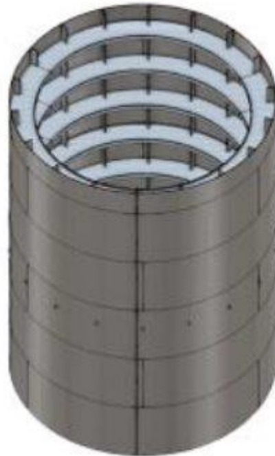
Tubular column with vertical & ring stiffeners
