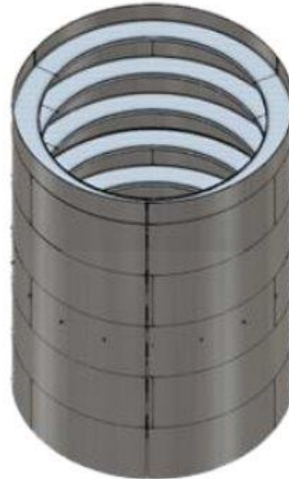
Tubular column with ring stiffeners
