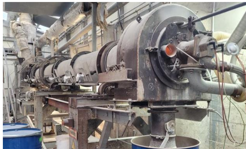
Rotary Kiln Calciner ( \approx 800^{\circ}\text{C} for 30 mins)
