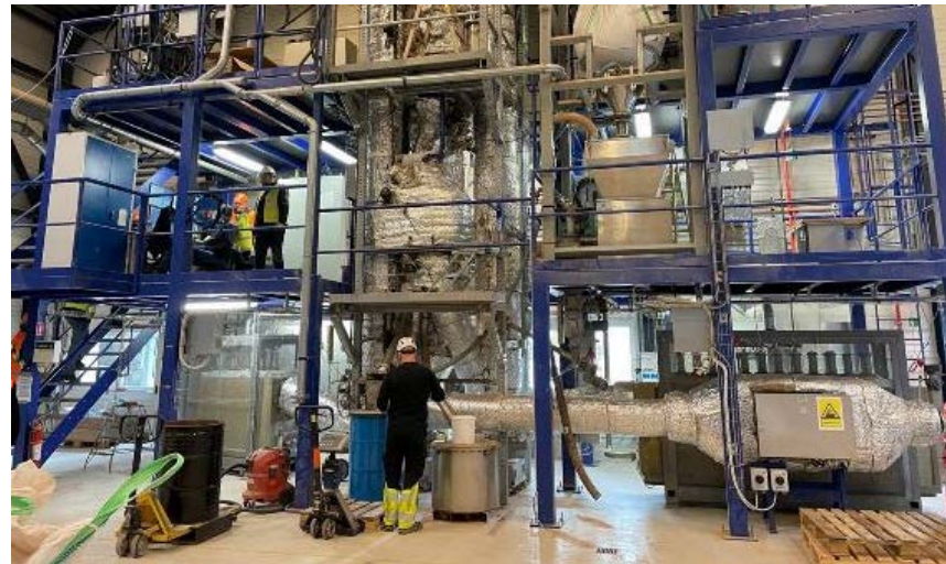
Flash Calciner ( \approx 850^{\circ}\text{C} for minutes)
